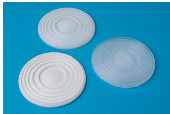
*Fig. 1. Monochromatic Fresnel lenses from various thermoplastic materials (COC, PLA, HIPS)*
