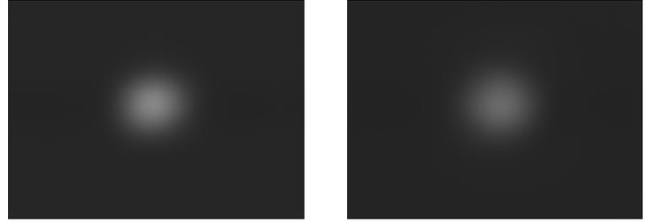
Fig. 4. Raw pictures of the intensity distribution of radiation focused by a monochromatic THz Fresnel lens (left) and refractive lens (right).
