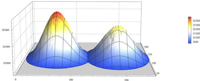
Fig. 3. Intensity profile of a beam focused by a monochromatic THz Fresnel lens (left) and refractive lens (right).
