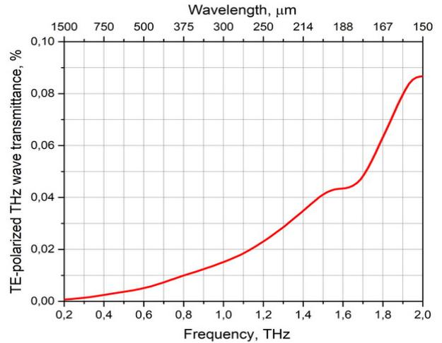
Fig. 2. Transmission of non-desired polarization, %
