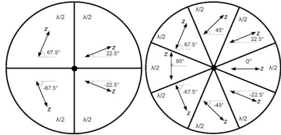
Operating principle of segmented waveplates:
