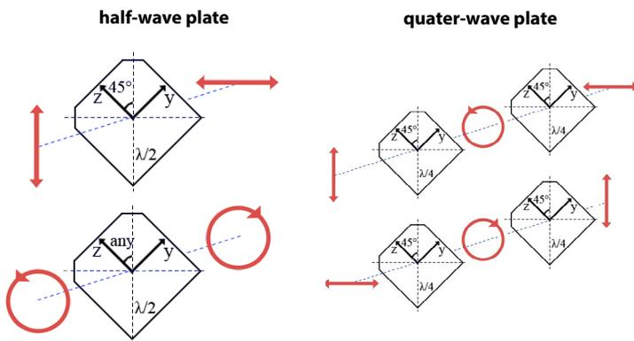
Tydex offers the THz waveplates for single operation wavelength.
