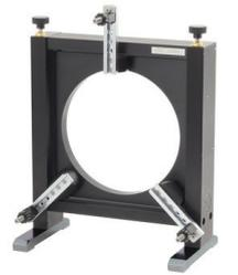
To hold large-size mirrors greater than 500 mm in diameter, we have developed a special rotating mount. When locking screws are loosened, the mount allows full 360° rotation of the mirror around horizontal and vertical axes.
