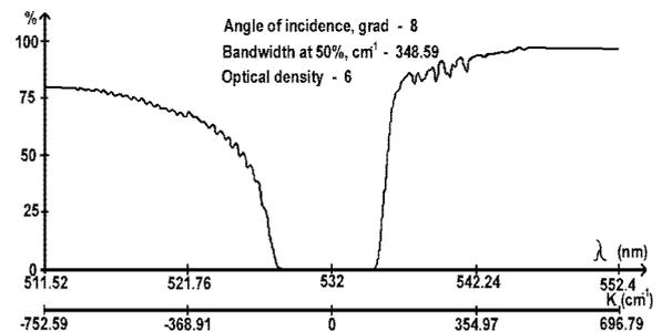
Fig.1 Typical transmission curves of the Notch-4 filter for 633 nm and Narrow Notch-6 filter for 532 nm
