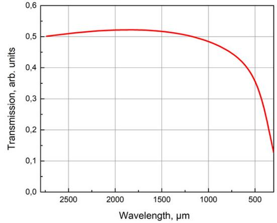
Fig. 3. Transmission spectrum of a 40 mm thick f-theta lens along the axis
