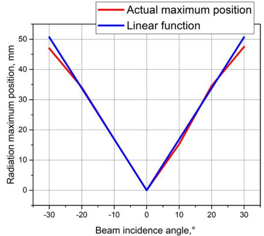
Fig. 4. Linearity of the f-theta lens characteristics
