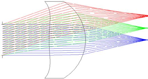
Fig. 1. THz aspherical f-theta lens
