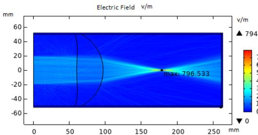
Fig. 2. Spatial distribution of electric field strength of a THz beam focused by an f-theta lens
