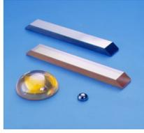
Tydex supplies custom ATR components in several geometries: trapezoids, parallelograms, rods, and hemispheres. Various materials are used: ZnSe, Ge, Si, and sapphire. All materials and products meet strict control standards including spectral characteristics and general performance requirements together with the specification control.
