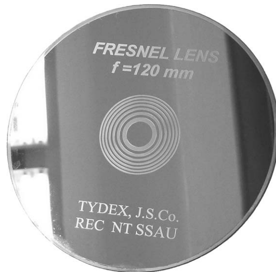
Fig. 3. Appearance of the binary diffractive lens.
