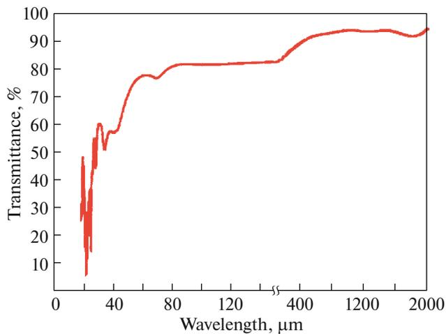
**Fig. 12.** (Color online) Transmission of a TPX window with a thickness of 2 mm in the THz range [23].
