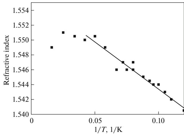
**Fig. 16.** Temperature dependence of the refractive index of HDPE [23].
