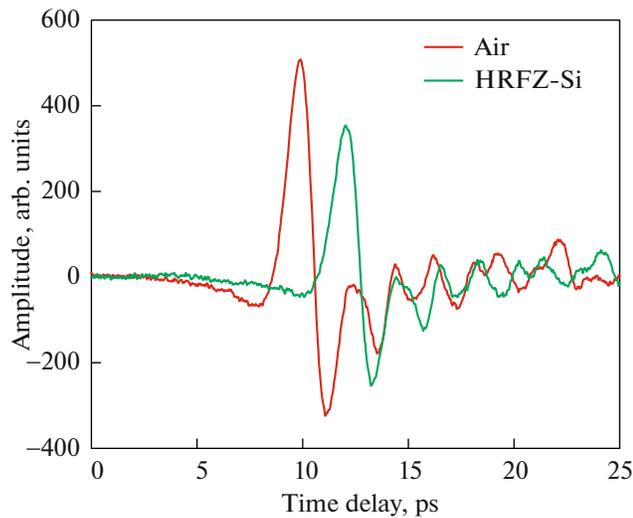
**Fig. 3.** (Color online) THz signals passed through the air and high-resistance silicon [23].
