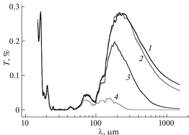
**Fig. 5.** Optical transmission of single crystals of (1) undoped germanium and (2–4) germanium doped with antimony; the resistivity values are as follows: (2) 46, (3) 20, and (4) 5 Ohm cm [39].
