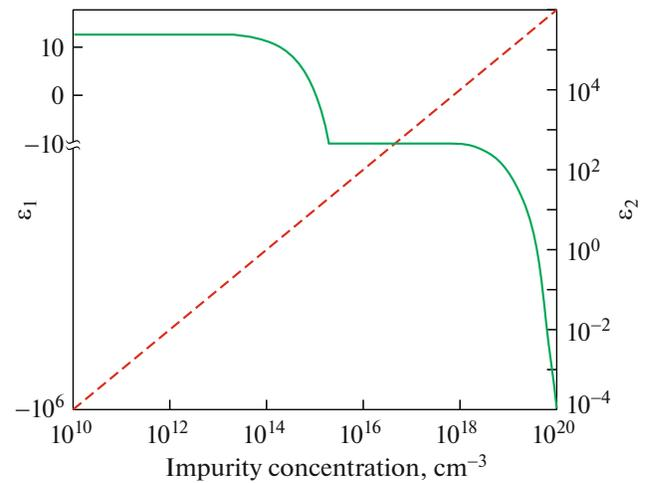
**Fig. 4.** (Color online) The real ( $\epsilon_1$ , solid line) and imaginary ( $\epsilon_2$ , dashed line) parts of the dielectric permittivity of silicon with different concentration of free carriers at a frequency of 1 THz [23].
