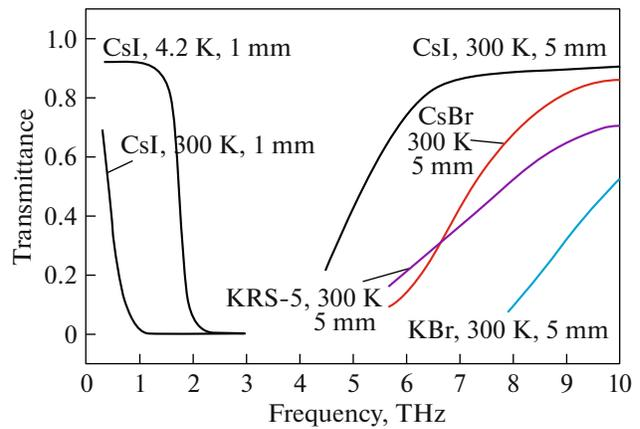
**Fig. 11.** (Color online) Optical transmission of halides at temperatures of 4.1 and 300 K [2].
