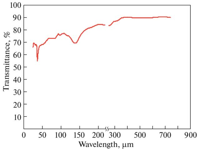
**Fig. 15.** (Color online) Transmission of a HDPE window with a thickness of 2 mm in the THz range [23].
