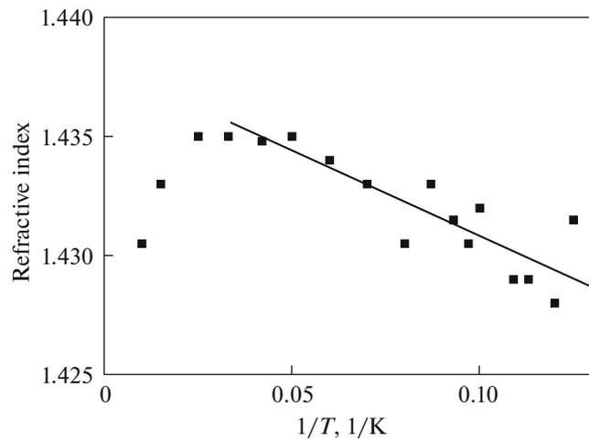
**Fig. 13.** Temperature dependence of the refractive index of TPX [23].
