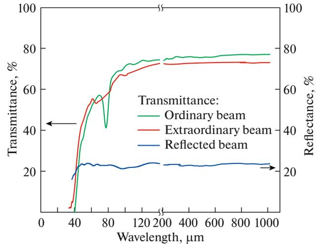
**Fig. 8.** (Color online) Transmission of a crystalline quartz sample with a thickness of 1 mm [44].
