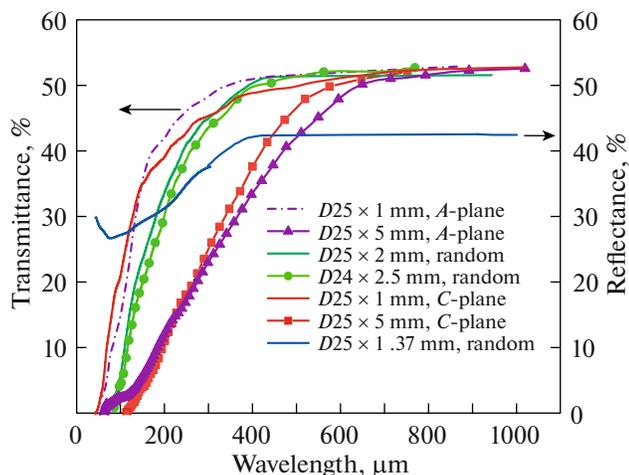
**Fig. 9.** (Color online) Transmission of sapphire samples of different thicknesses and crystallographic orientation [46].
