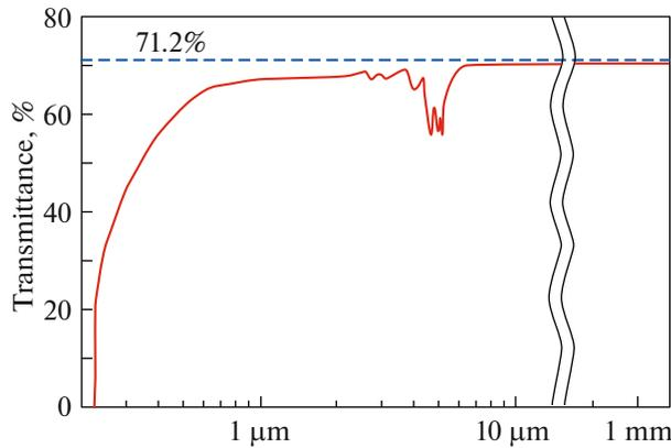
**Fig. 10.** (Color online) Transmission spectrum of a 1 mm thick PD plate [25].
