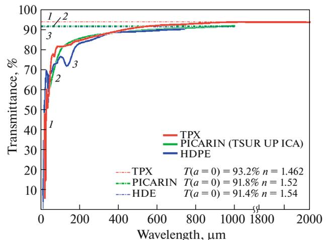
**Fig. 14.** (Color online) Transmission of samples of TPX, picarin, and HDPE (high density polyethylene) [23].
