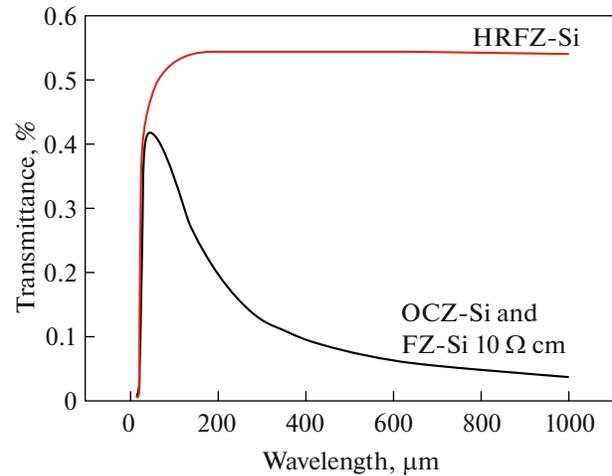
**Fig. 2.** (Color online) Transmission of silicon in the range 16–1000  $\mu\text{m}$ ; the thickness of samples is 5 mm [29].
