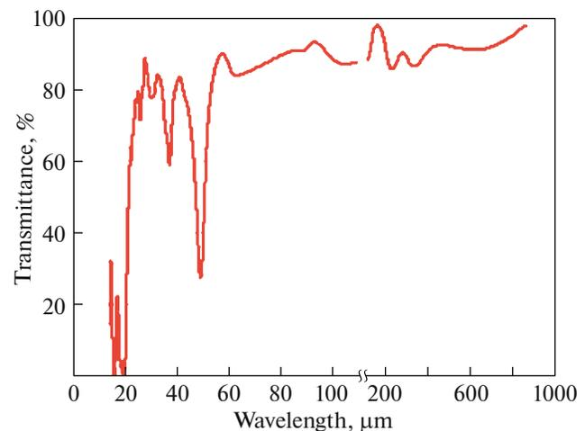
**Fig. 17.** (Color online) Transmission of a PTFE film with a thickness of about 0.1 mm in the THz range [23]
