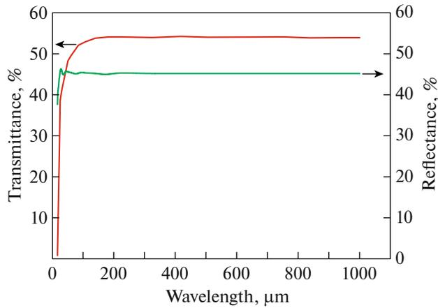
**Fig. 1.** (Color online) Transmission and reflection of high-resistance silicon with a thickness of 1 mm in the THz range [29].
