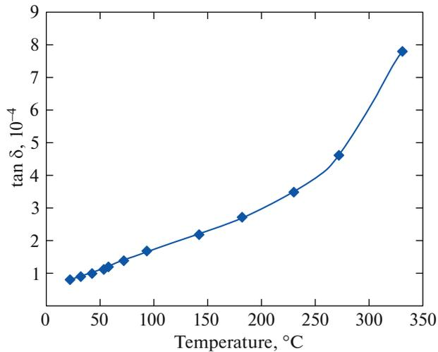
**Fig. 7.** (Color online) Temperature dependence of the  $\tan \delta$  value in the temperature range 20–350°C [41].
