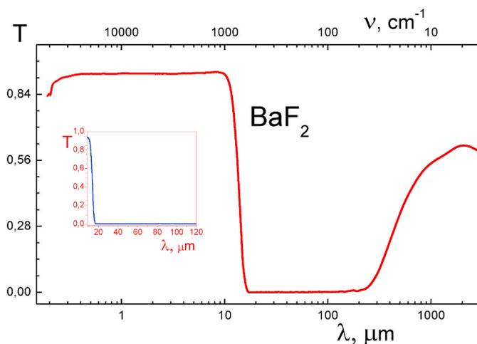
Fig. 5. The spectral dependence of the transmission of  $\text{BaF}_2$  crystal with a thickness of 2 mm.
