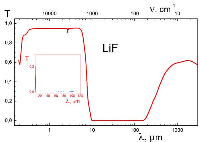
**Fig. 2.** The spectral dependence of the transmittance of LiF crystal with a thickness of 2 mm.
