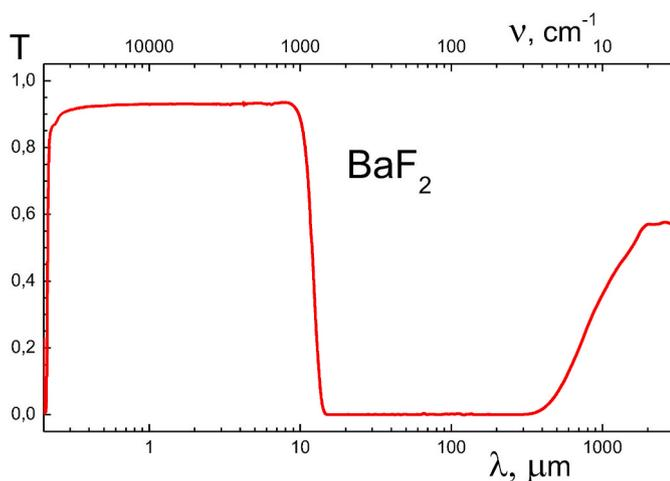
Fig. 6. The spectral dependence of the transmission of  $\text{BaF}_2$  crystal with a thickness of 7.29 mm.
