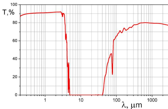
Fig. 7. Transmission spectrum of crystalline quartz Z cut.
