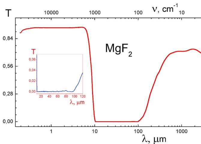
Fig. 4. The spectral dependence of the transmission of  $\text{MgF}_2$  crystal with a thickness of 2 mm.
