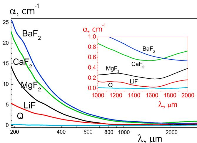
Fig. 8. Calculated spectra of attenuation coefficients for single crystals of LiF, CaF<sub>2</sub>, BaF<sub>2</sub>, MgF<sub>2</sub> and crystalline quartz (Z cut) in the range 200–3000 μm.
