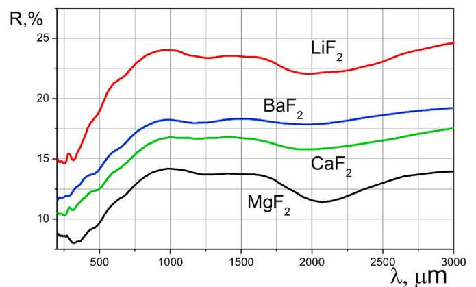
**Fig. 1.** Reflection spectra of fluorides of magnesium, lithium, calcium and barium in the THz range.
