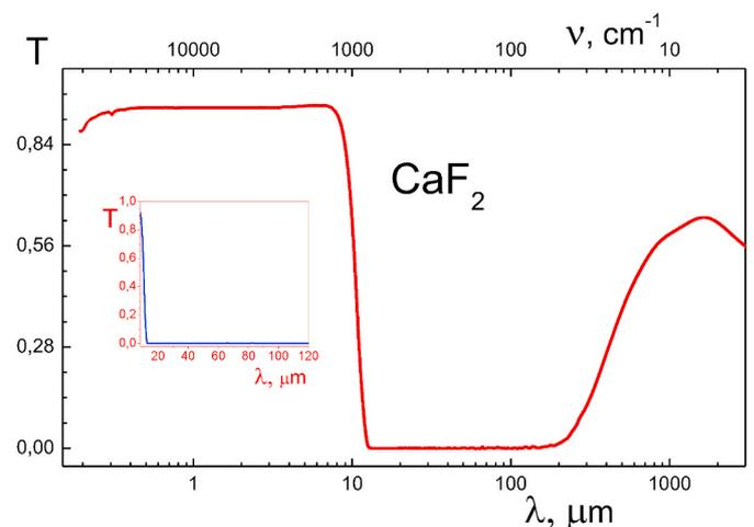
**Fig. 3.** The spectral dependence of the transmittance of CaF<sub>2</sub> crystal with a thickness of 2 mm.
