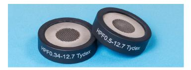
THz High pass filters (HPF) are designed to block lower frequencies and allow only high terahertz frequencies to pass. The filters are made from metal plates with subwavelength diameter holes. The plates are mounted in holders with fit rings. The micro-sized holes in the filters act as waveguides with reject frequency determined by the hole geometry.
